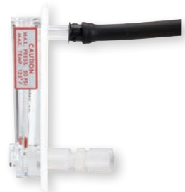
Model MMF connections. Connector at top, installed in panel, has retainer and flexible tubing in place. Connector at bottom shows alternative connection with metal or rigid plastic tubing, using a double compression nylon tube union (as Dwyer Part No. A-328).
