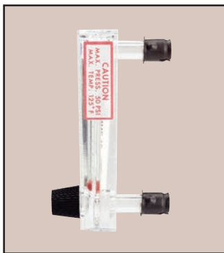
Model MMF mounts easily from front of panel. Drill two 9/32" or 5/16" dia. holes in panel on 2-1/16" centers. Insert mounting connector spuds. From rear, slide on the two spring retainers (furnished) and push on rubber or plastic tubing.
