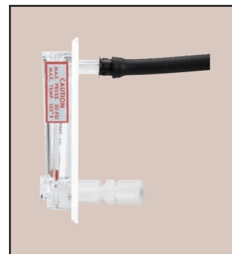
Model MMF connections. Connector at top, installed in panel, has retainer and flexible tubing in place. Connector at bottom shows alternative connection with metal or rigid plastic tubing, using a double compression nylon tube union (as Dwyer Part No. A-328).
